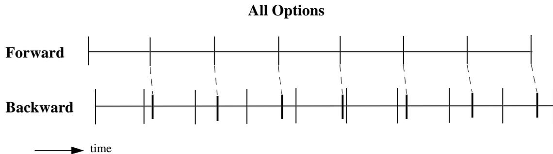
Vertical lines represent RM-cells. Longest lines are forward RM-cells. Middle length lines are in rate backward RM-cells. Shortest lines are out of rate backward RM-cells. All vertical lines on the forward links represent forward RM-cells.
