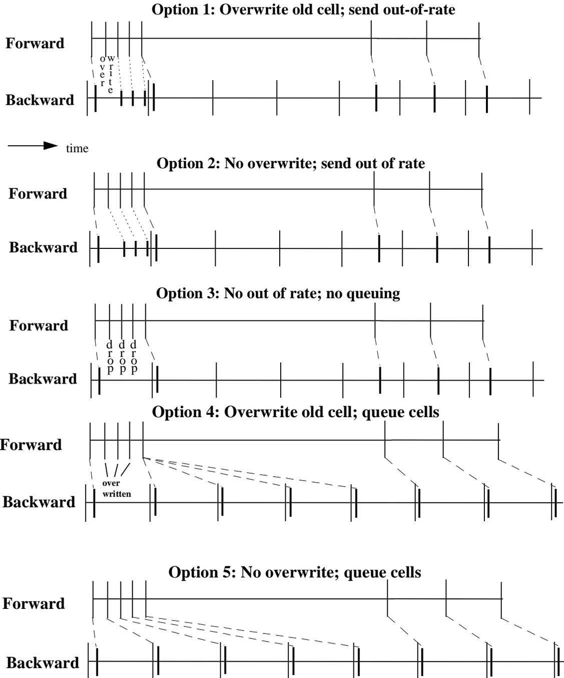
Notice that the difference between options 4 and option 5 is that option 4 always uses the latest received forward RM-cell's contents while option 5 keeps the older RM-cells' contents in the queue. The queue of option 4 could be implemented with a counter along with a single RM-cell storage area. Option 5 requires a storage area for each of the queued RM-cells.
