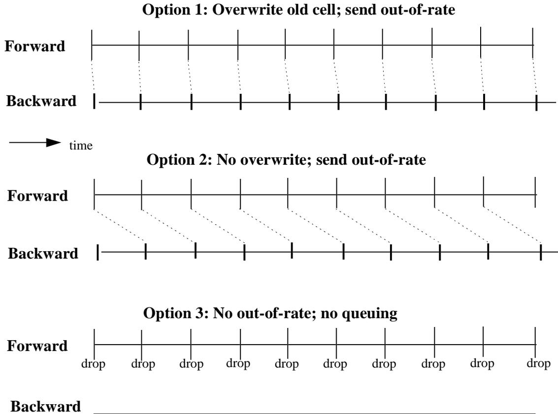
In this case, since there are no in-rate slots in the backward direction, both option 1 and option 2 send nothing but out-of-rate backward RM-cells. The only difference between these two options is in the latency of the out-of-rate backward RM-cell's contents. Option 1 transmits the newly arrived forward RM-cell's contents as the out-of-rate backward RM-cell and option 2 transmits the old forward RM-cell's contents as the out-of-rate backward RM-cell.
