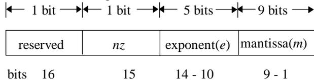
**Figure 5-4: Rate format used in RM-cells**
