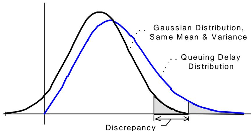
**Figure V-1: The discrepancy of a queuing delay density**
