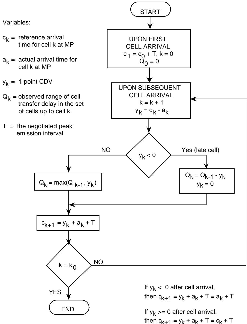
**Figure B-1: Estimation of the range of two-point CDV from one-point CDV for connections providing CBR service**
